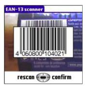
Barcode/13 is a full software barcode scanner for palmOne **Treo600** and palmOne **Treo650**. Barcode/13 uses the Treo camera to scan UPC-A and EAN-13 barcodes and exports the decoded value to the system clipboard. Barcode/13 can be launched within any application, and the returned value can be retrieve from the clipboard to make use of it into the initial application.
