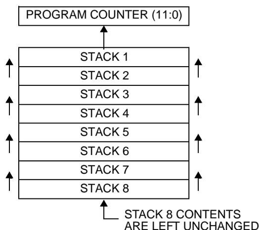
**Figure 2-6** Stack Operation for a “Return” Instruction
