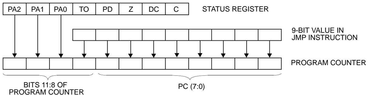
**Figure 2-3** Program Counter Loading for Jump Instruction
