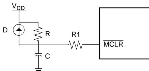
**Figure 4-8** External Power-On  $\overline{MCLR}$  Signal
