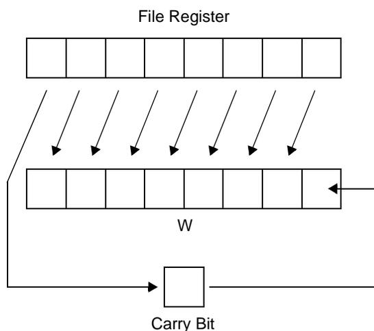
**Figure 3-2** Rotate fr Left Through Carry into W
