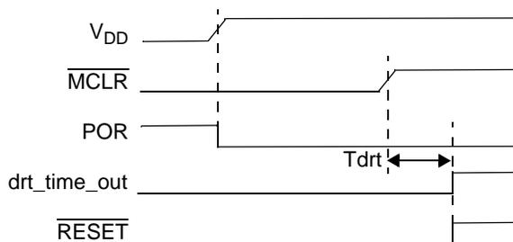
**Figure 4-9** Power-On Reset Timing, Separate  $\overline{MCLR}$  Signal
