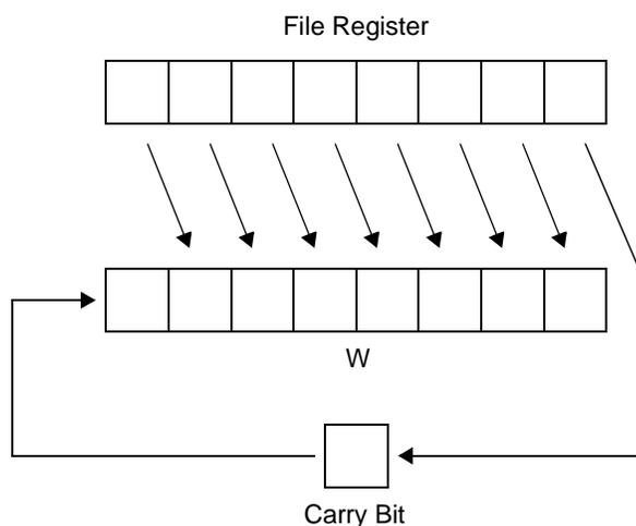
**Figure 3-3** Rotate fr Right Through Carry into W
