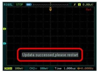
• unplug the USB memory stick, switch the DS1052E off. This completes the firmware downgrade.
