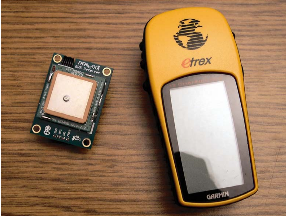
Figure 139.1: The Parallax GPS Module (left) and the Garmin eTrex GPS Unit (right)
